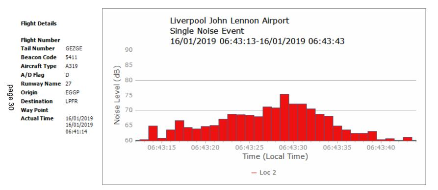
Example of a Noise Event Report form the Noise Monitoring System (NMT 2) for a easyJet Airbus A319 arrival on departure on runway 27.
